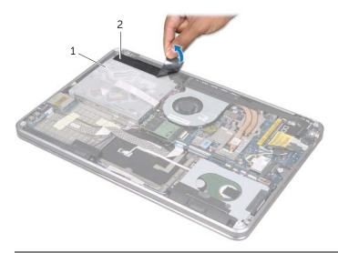
1 optical-drive assembly 2 mylar
